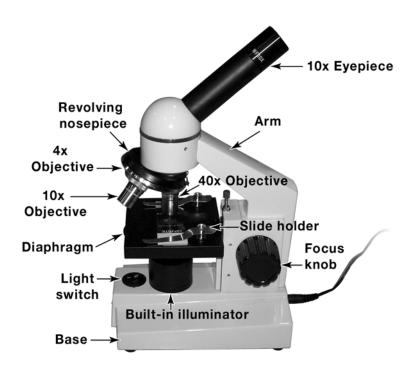
Look at the picture above. Each of the parts of the microscope is labeled. The major parts of the microscope are the light source, the specimen stage, the eye piece, and the objective lenses. You will find a description of the microscope parts at the end of this write up.
